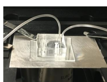
Microfluidic Flow System (NE-500X2) Microscope view of the H-Channel in a microfluidic chip PDMS Microfluidic Chip (Fluid-Flow Testing)
