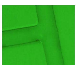
Microfluidic Flow System (NE-500X2) Microscope view of the H-Channel in a microfluidic chip PDMS Microfluidic Chip (Fluid-Flow Testing)
